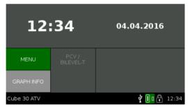
The standby screen shows the time and date in the top section. If the respiratory humidifier is connected, the set heating performance of the respiratory humidifier is displayed in this area. The heat level then works via the right/left keys.
