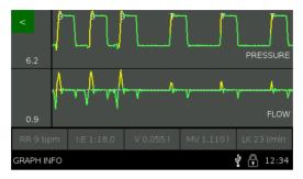
The current measured value is displayed on the left-hand side of each of the graphs.
