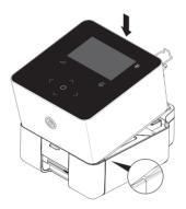
Connect the power mains cable to the device. Secure the power cable to the device with the help of the safety clip. Insert the other end of the mains cable into a socket.
