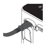
6. Connect the respiratory tube to the air outlet on the respiratory humidifier.
